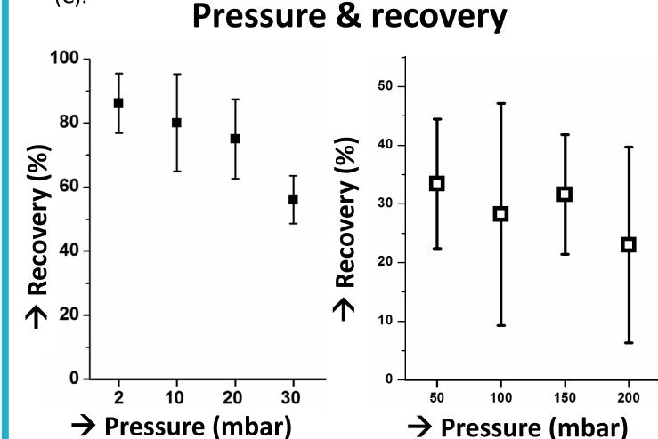
Figure 6: The relation between the pressure and recovery of 300 SKBR3 cells from 1 ml of unfixed whole blood using tracketched membranes (A) and 250 colo320 cells from 7.5 ml of cellsave fixed blood(B).
