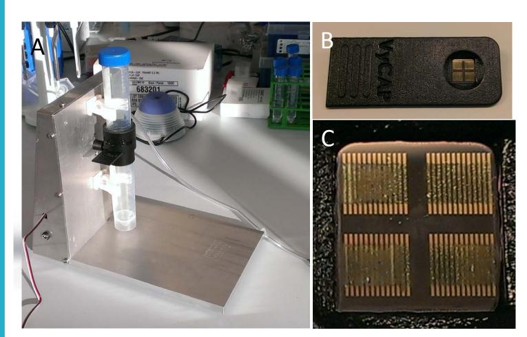
Figure 5: Collected Samples are filtered using a filtration station (A) which provides a fixed pressure across a silicon nitride filter mounted in a slide (B) with >100.000 5um pores
