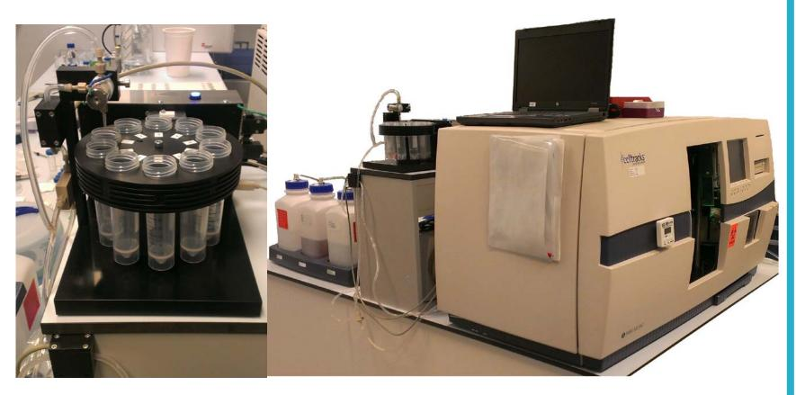
**Figure 4:** The automated station for the collection of discarded blood samples from the CellSearch AutoPrep waste line.
