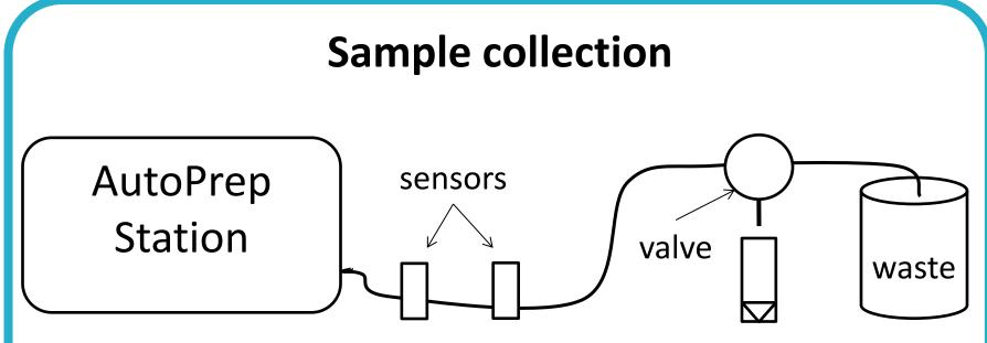
**Figure 3:** Schematic overview of the collection of discarded blood from the CellSearch System. Sensors detect the approach of a sample and valve is operated to transfer it to a 50ml conical tube.
