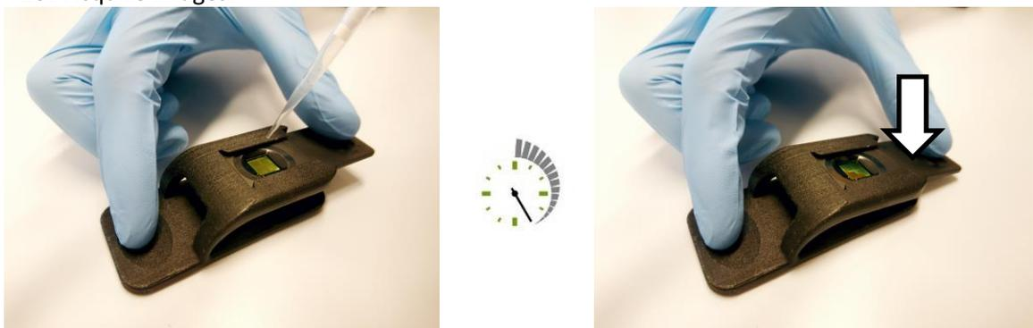
**Figure 2:** Permeabilization, washing, staining and fixation of the cells are all performed using the sieve staining holder. Solutions can be applied directly on the sieve (left). The solution will stay on the sieve during incubation. By gently pushing down the end of the slide, the sieve will come in contact with the absorber underneath and this will absorb the solution (right).
