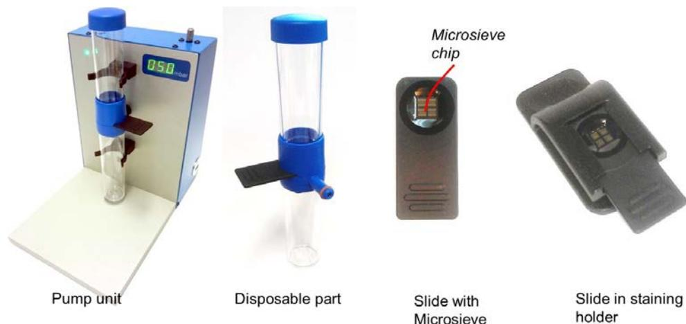
Figure 1: Filtration components.
